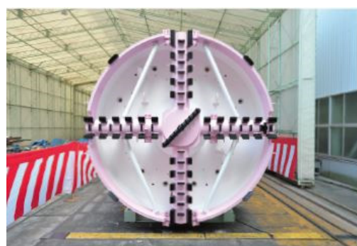
A dia. 4.48m earth pressure balance shield tunneling machine
