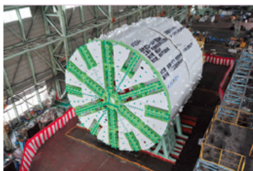
Shield tunneling machines for Yokohama Ring Expressway North-West Line (diameter 12.64 m)
