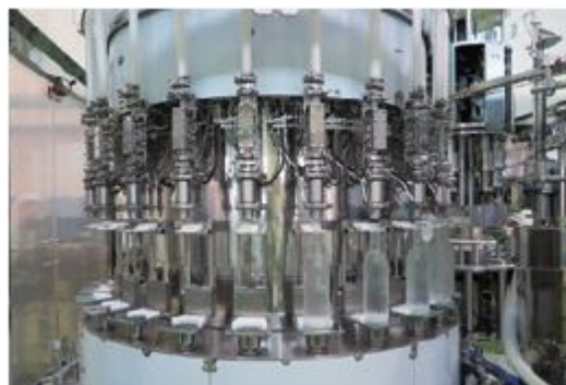
Filling system for amazake sweet fermented rice drink with a magnet-driven shutter-nozzle (newly developed)
