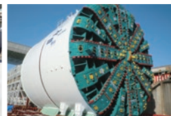
● Shield tunneling machines
