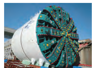
● Shield tunneling machines
