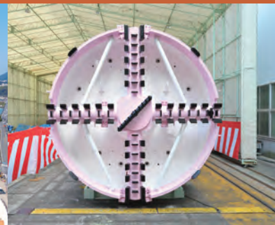
A dia. 4.48m earth pressure balance shield tunneling machine
