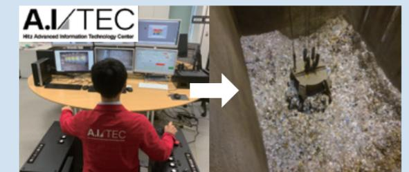
Remote operation of the waste crane from A.I./TEC.
