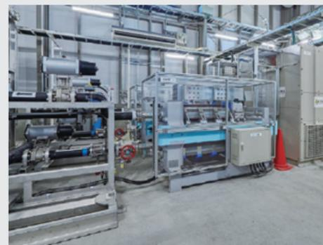
Hydrogen generation system for Hokkaido Electric Power Co., Inc.
