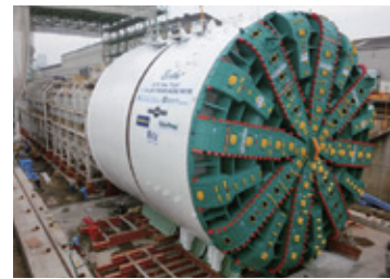
Shield tunneling machine
