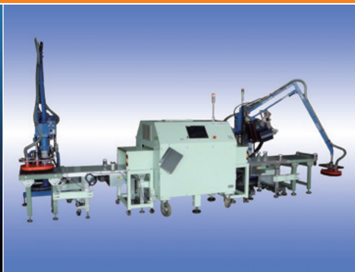
Belt conveyor radiation screening system
