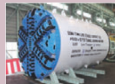
Shield tunneling machine for construction of subway line in Singapore
