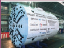
Shield tunneling machine for use in construction of tunnel under the Bosphorus Strait in Istanbul, Turkey
