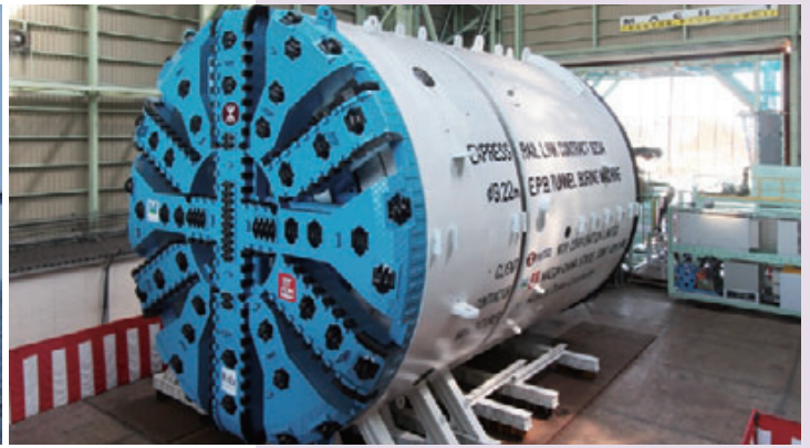
Shield tunneling machine for Hong Kong super-express railway tunnel
