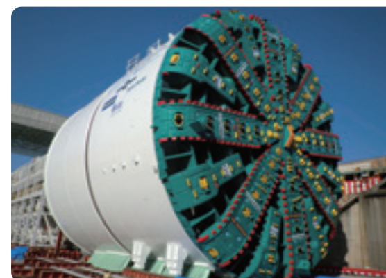
17.45m diameter earth pressure balance Shield Tunneling Machine for the city of Seattle, USA.
