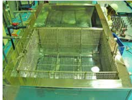
精密部品洗浄装置 (超音波洗浄機) Precision Parts Cleaning Equipment (ultrasonic washing machine)
