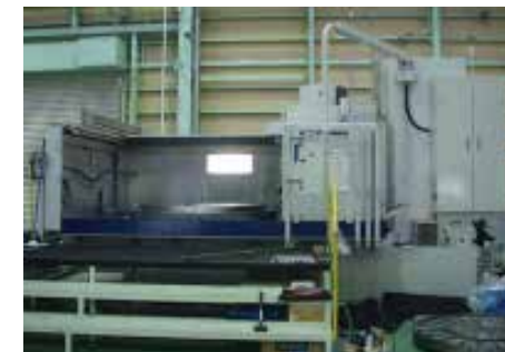
立軸円テーブル形平面研削盤 Vertical Spindle Rotary Surface Grinding Machine
