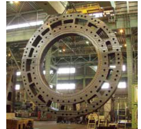
原子炉ペDESTAL(基礎) Pedestal of nuclear reactor (basement)
