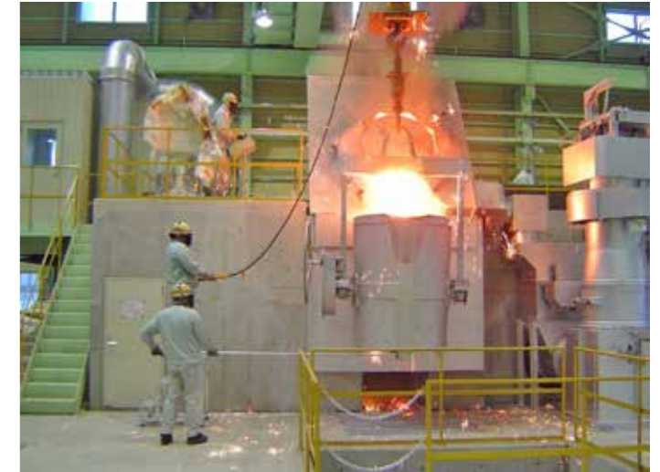
鋳造工場での鋳込みのための出湯作業風景 A scene of the work of the dye for casting in the casting worksite
