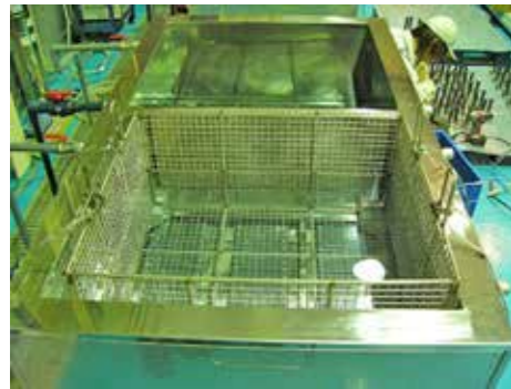
精密部品洗浄装置 (超音波洗浄機) Precision Parts Cleaning Equipment (ultrasonic washing machine)
