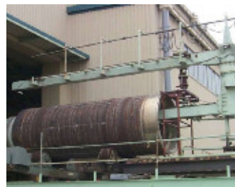
γ線遮へい性能検査設備 Inspection equipment for gamma ray shielding performance
